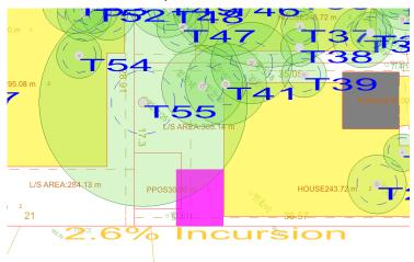
This modification will reduce the encroachment from 7.2% to 2.6%. Further reduction may be achieved by utilizing pier and beam technology with the remaining PPOS located inside the TPZ, this would result in approximately 0.5% incursion.
