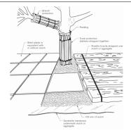
Figure 4 - Trunk, Branch & Ground Protection
