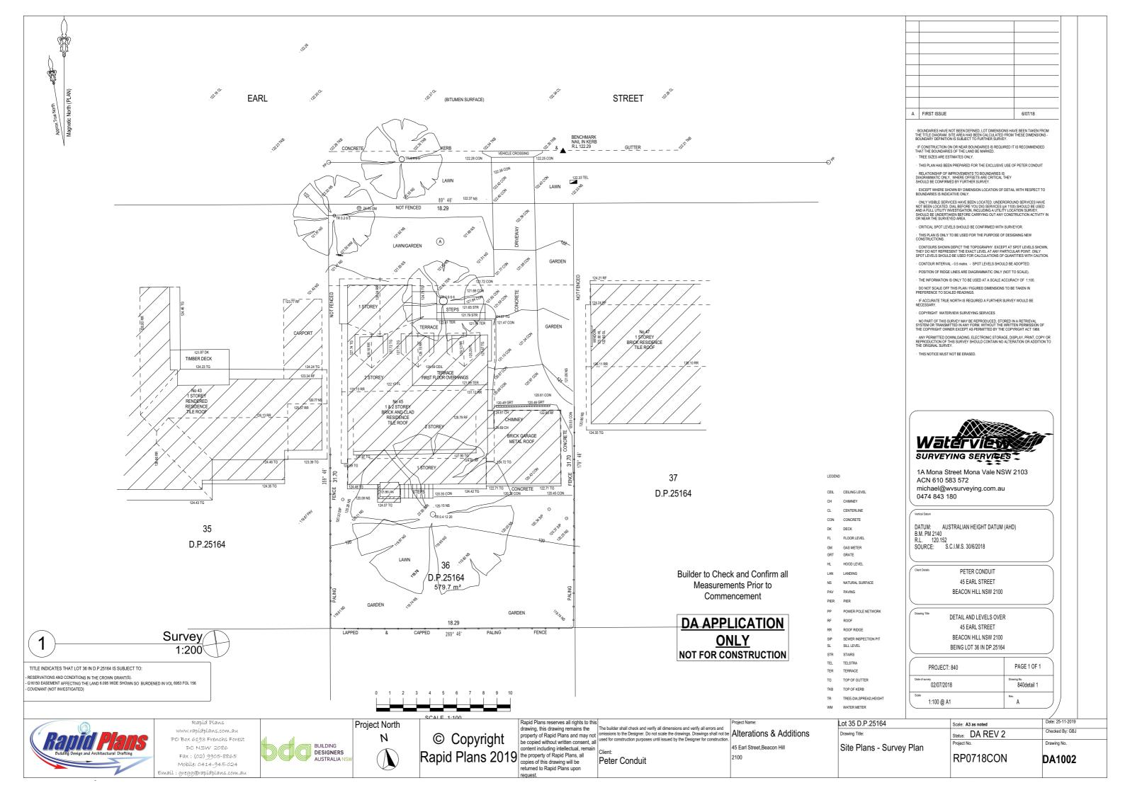
BENCHMARK NAIL IN KERB R.L 122.29 CONCRETE/ VEHICLE CROSSING TR-0.4 6 5 122.28 CON 122.25 CON 89° 46' 122.37 NS NOT FENCED 18.29 LAWN/GARDEN GARDEN 121.72 CON 121.68 CON STEPS 121.65 STR , 121.79 STR 121.47 CON 121.94 TER GARDEN CAŔPORT 1 STOREY BRIOK RESIDENCE TILE ROOF 121.87 DK TIMBER DECK 124.23 TG No 43 1 STOREY RENDERED RESIDENCE TILE ROOF 120.61 CON 120.49 GRT 120.49 GRT 1 & 2 STOREY
