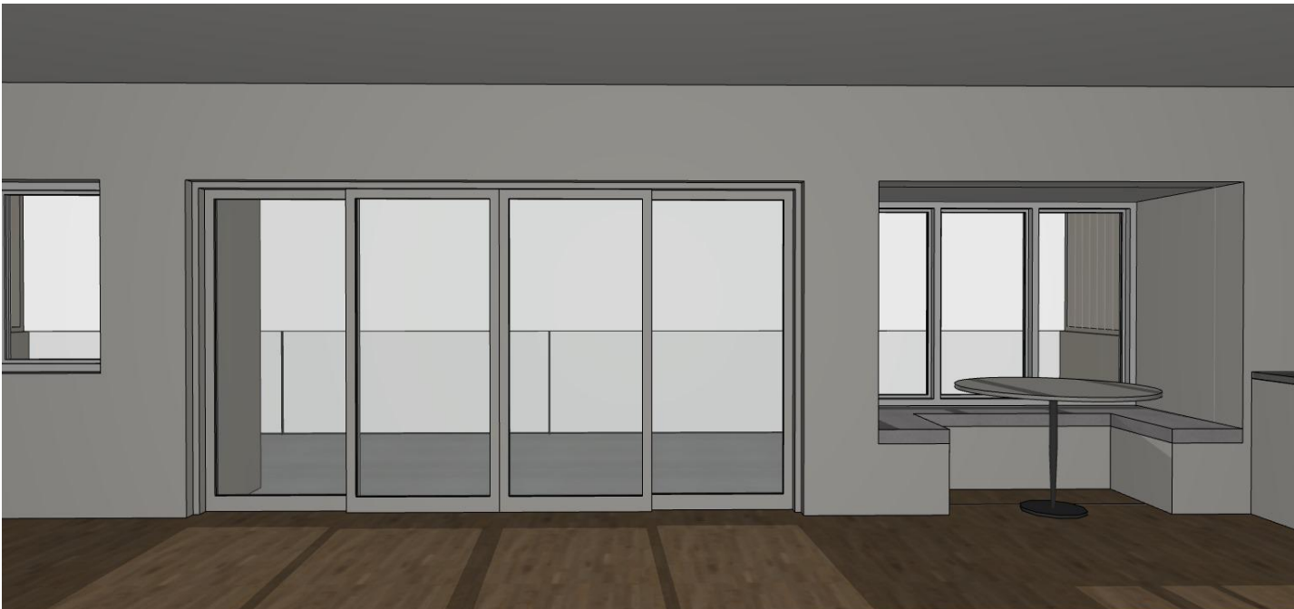
BAY WINDOW AND SLIDING DOOR
