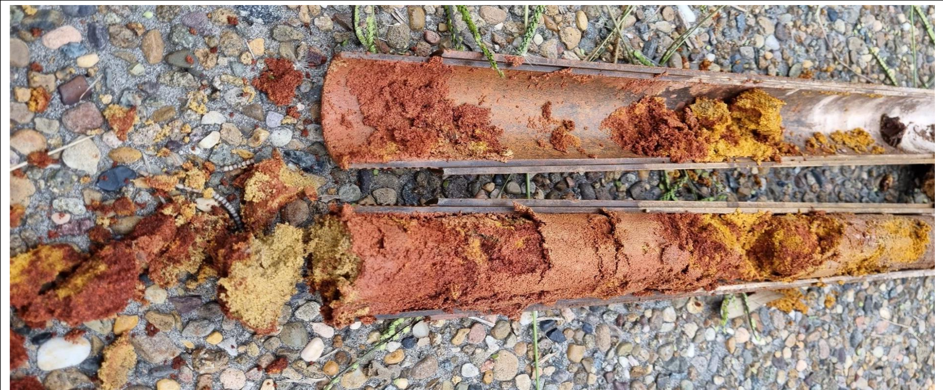
Figure 2.3 – Detail View of SPT Recovered Material (1.0m blg)
