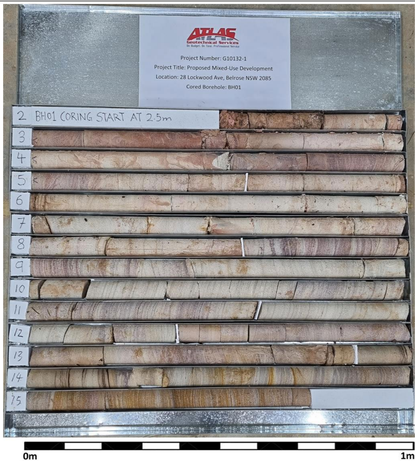
Figure 3.1 – Borehole 1 Core Specimens
