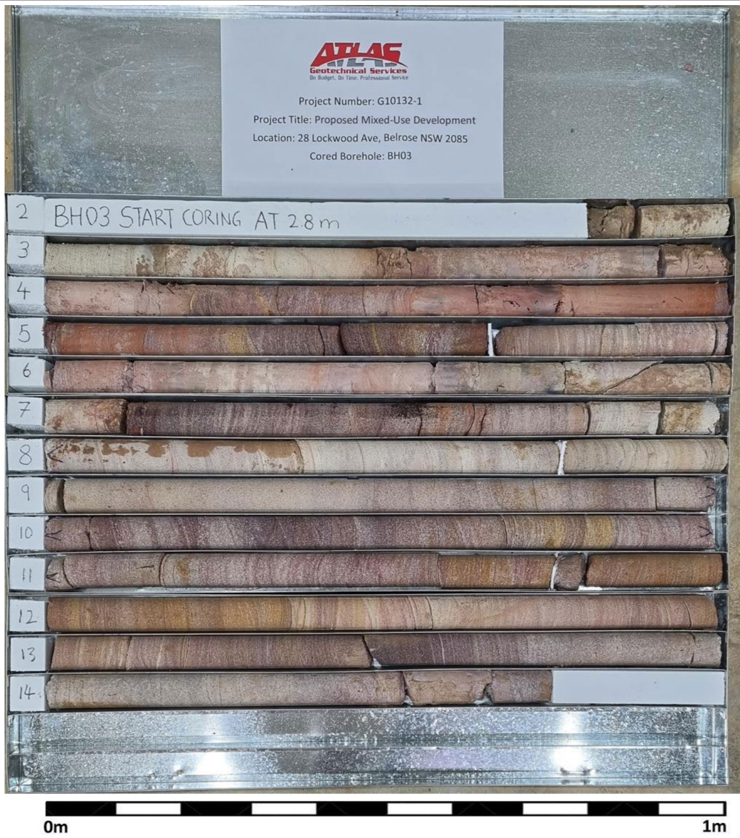
Figure 4.1 – Borehole 3 Core Specimens
