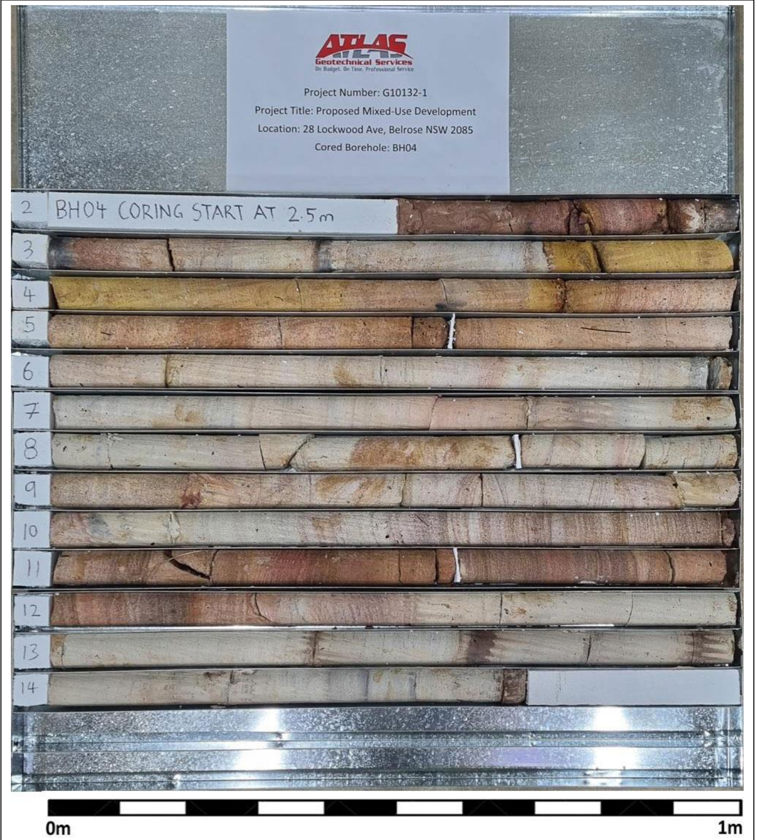
Figure 4.2 – Borehole 4 Core Specimens
