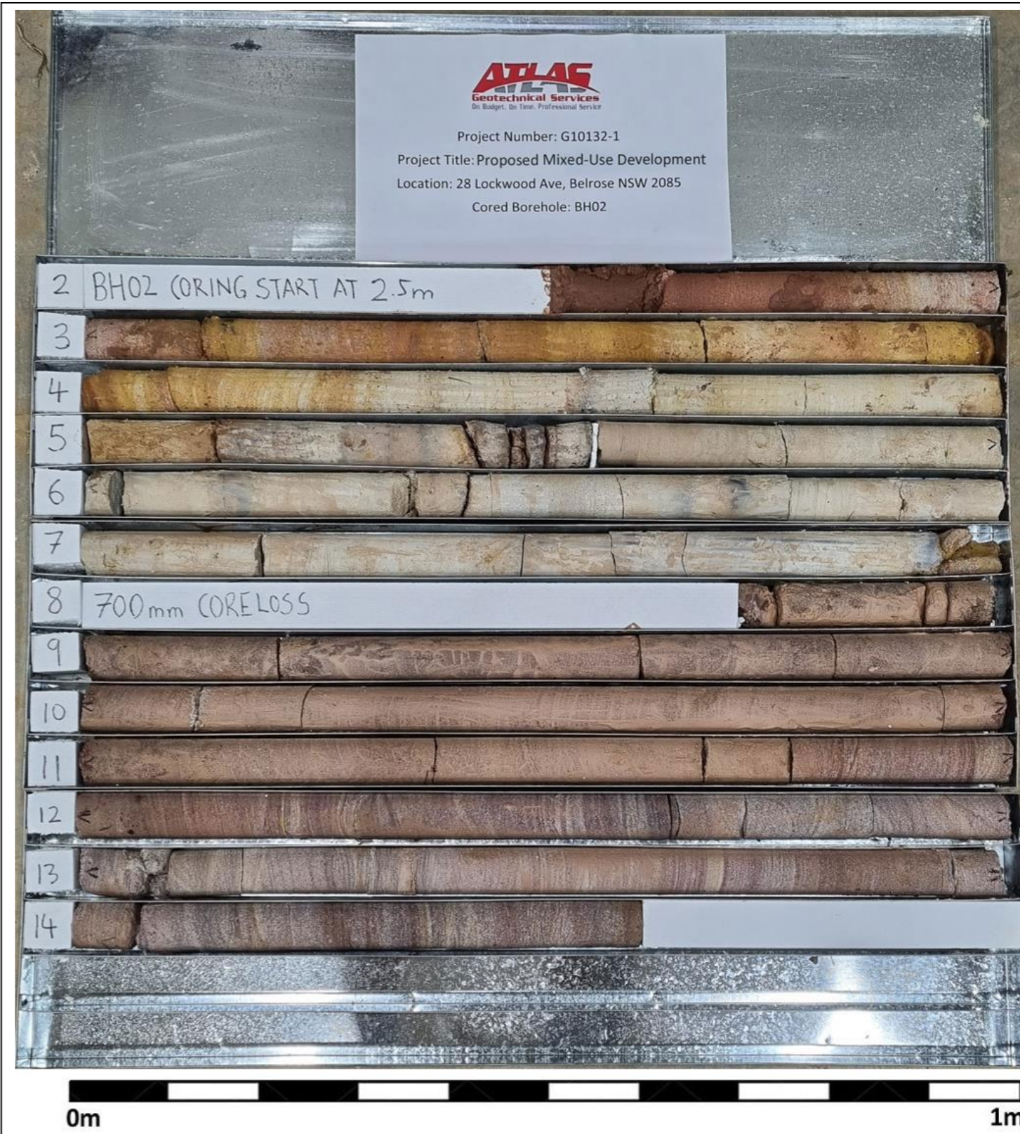
Figure 3.2 – Borehole 2 Core Specimens
