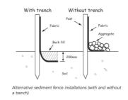
TYPICAL SEDIMENT FENCE DETAIL - N.T.S
