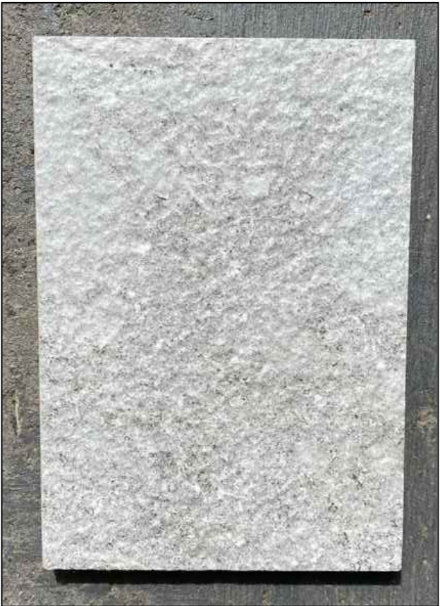
example of 600x300 vitrified floor tile for balcony and proposed new enclosed room on existing balcony (non slip finish for external area tile)
