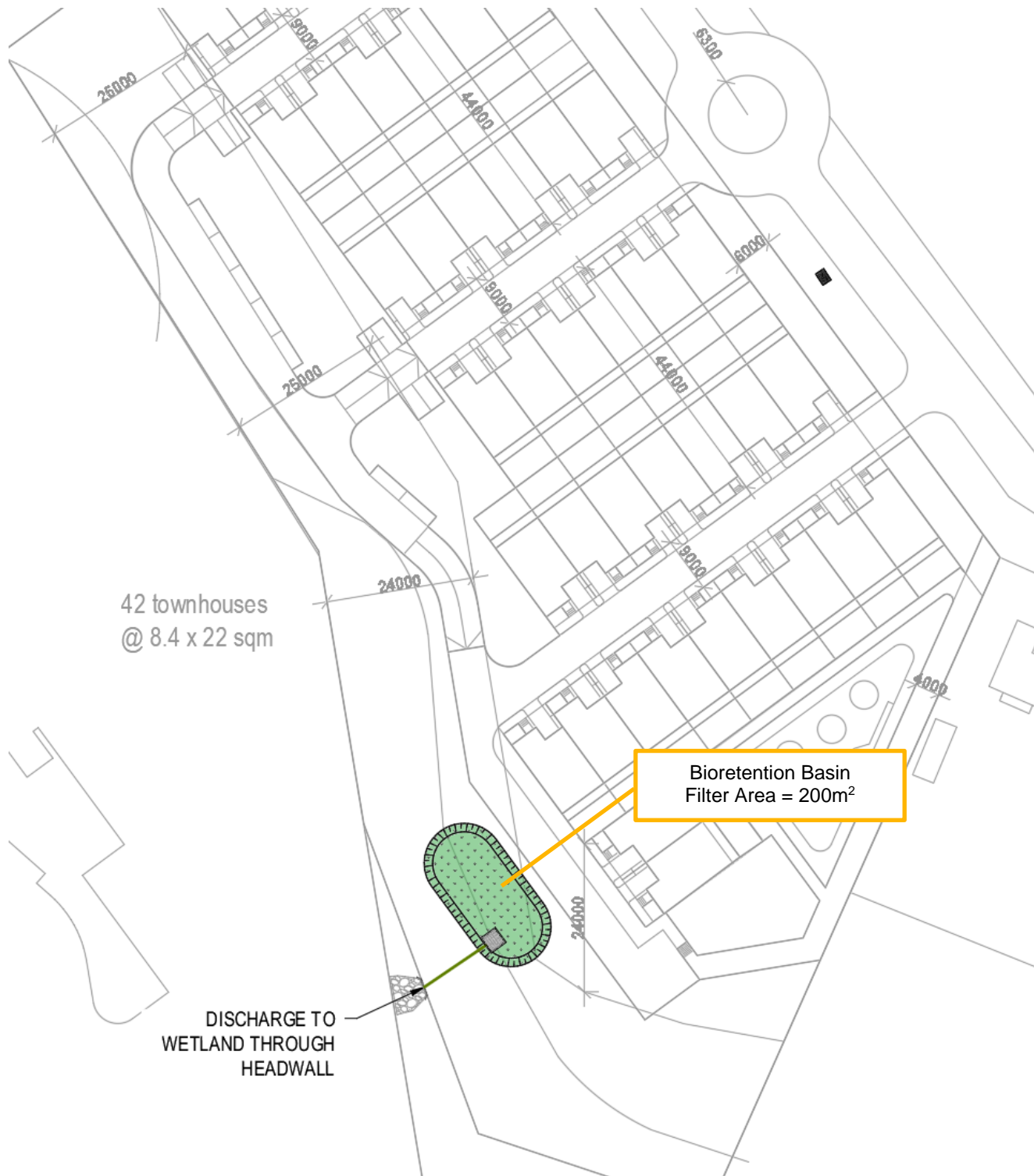
Figure 9: Tentative Location of Bioretention Basin
