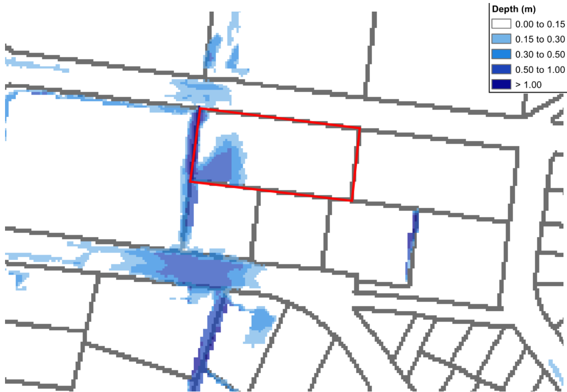
Figure 3 - 1% AEP Flood extent.
