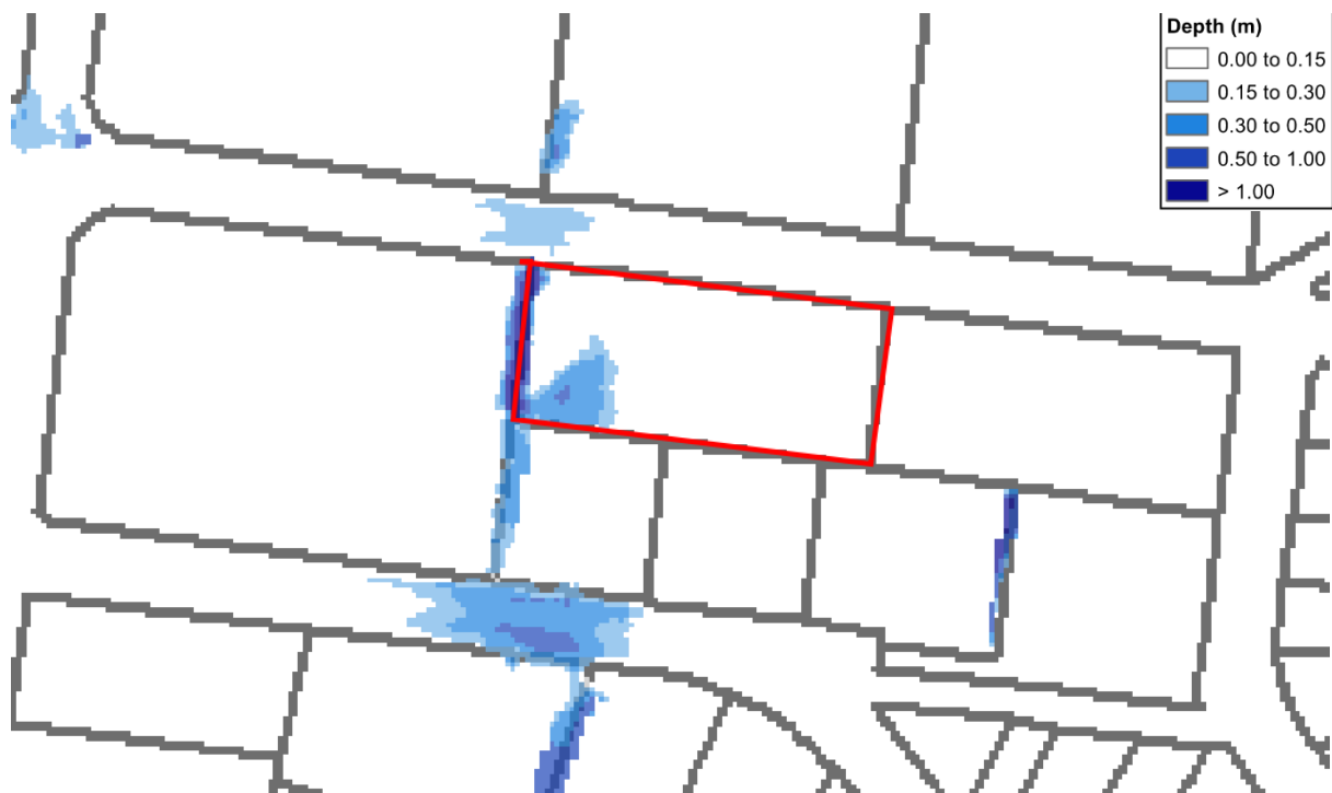
Figure 2 - 20% AEP Flood extent.
