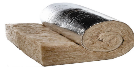
KNAUF EARTHWOOL ROOFING BLANKET WITH FOIL FACING 55mm THICK TO COMPLY WITH THE 'BASIX' CERTIFICATE No.A416055
