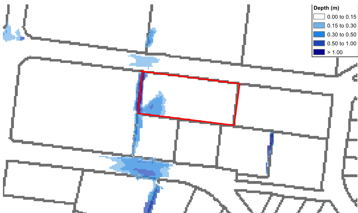
Figure 3 - 20% AEP Flood extent
