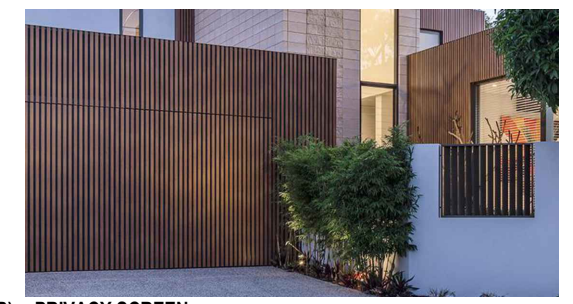
(B) PRIVACY SCREEN CHARRED TIMBER COLOURED POWDER COATED ALUMINUM PRIVACY SCREENS TO COMPLY WITH BAL-FZ REQUIREMENTS OR SIMILAR TO MATCH EXISTING. COLOUR TO BE DARK AND EARTHY TONED AS PER DCP REQUIREMENTS.
