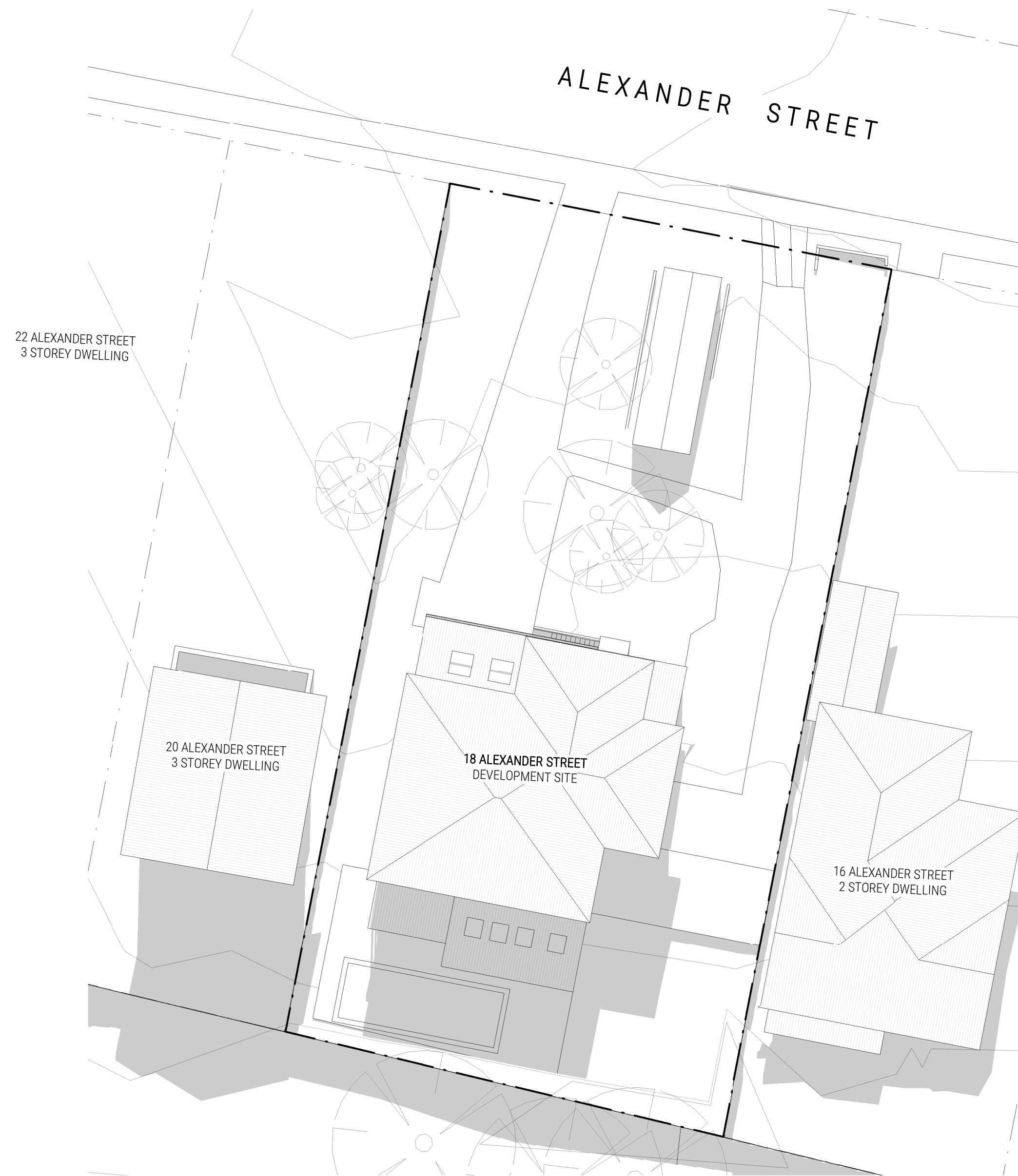
1 EXISTING SHADOW DIAGRAM - 12PM JUNE 21ST DA502/ 1:200 @ A1
