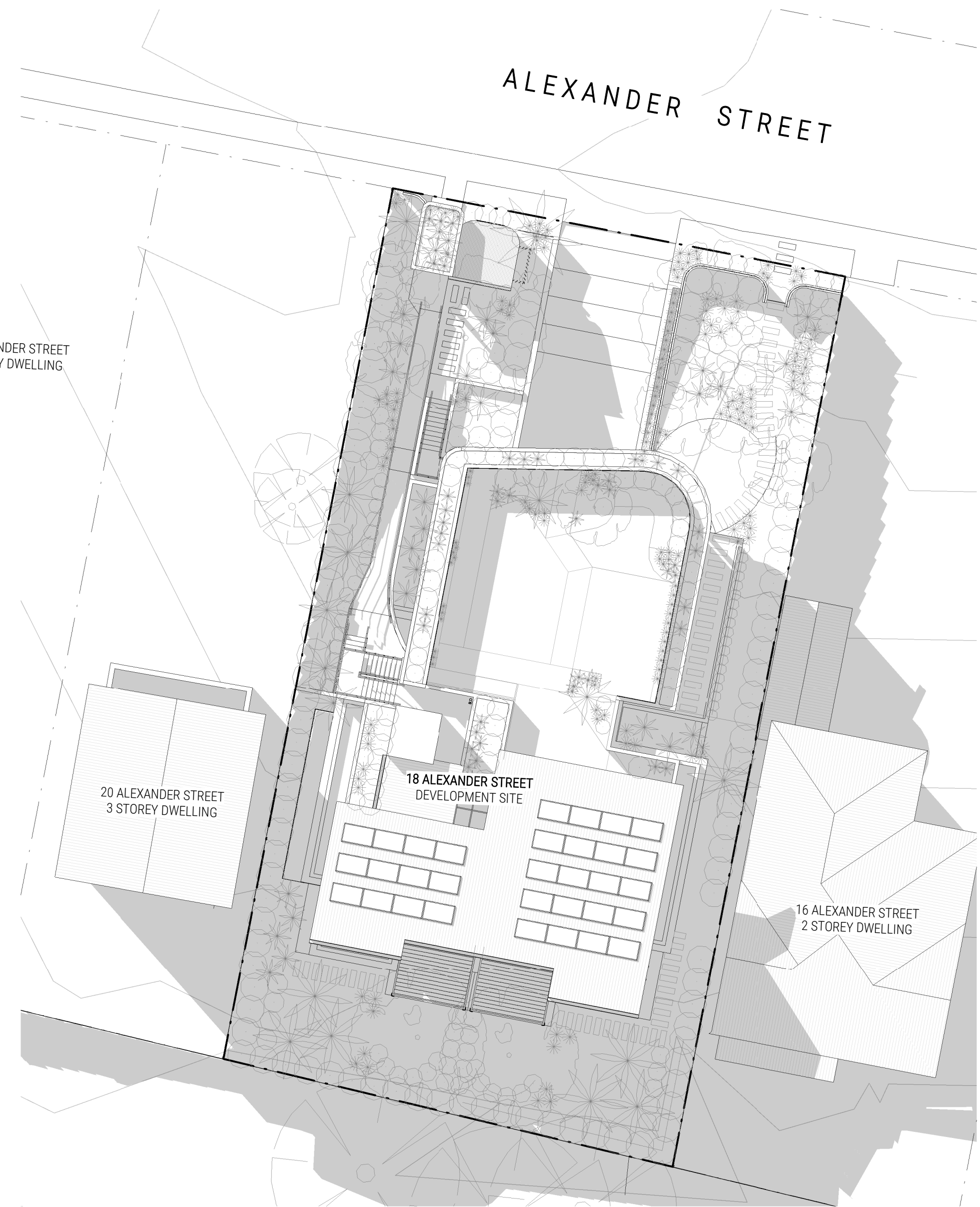
2 PROPOSED SHADOW DIAGRAM - 3PM JUNE 21ST DA503/ 1:200 @ A1
