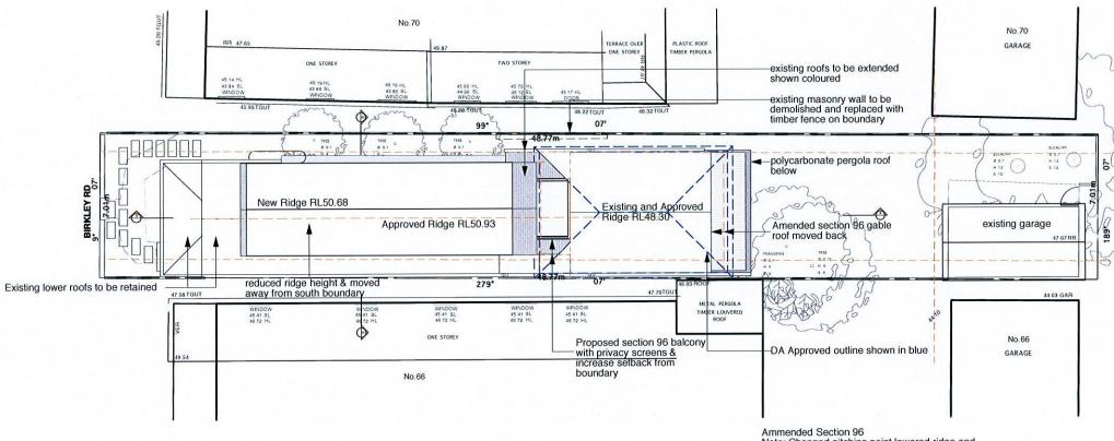
Ammended Section 96 Note: Changed pitching point lowered ridge and relocated ridge away from boundary. Reduced roof overhang to upper & lower floor gable roof on east side.
