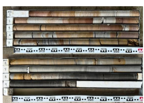
Photo 2: Bore Hole 2 core sample
