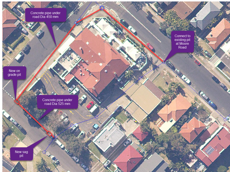
Figure 9: Option 2. Pipe diverted around the subject area from Undercliff Road to Moore Road
