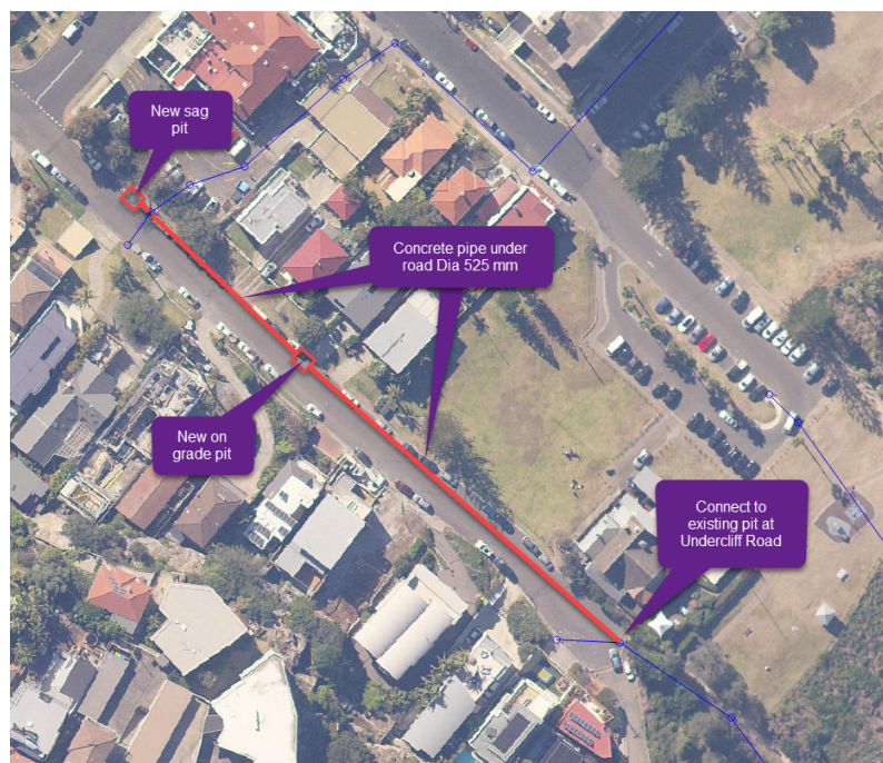
Figure 5: Option 1. Pipe connected through Undercliff Road to downstream council and discharge to the Freshwater Beach
