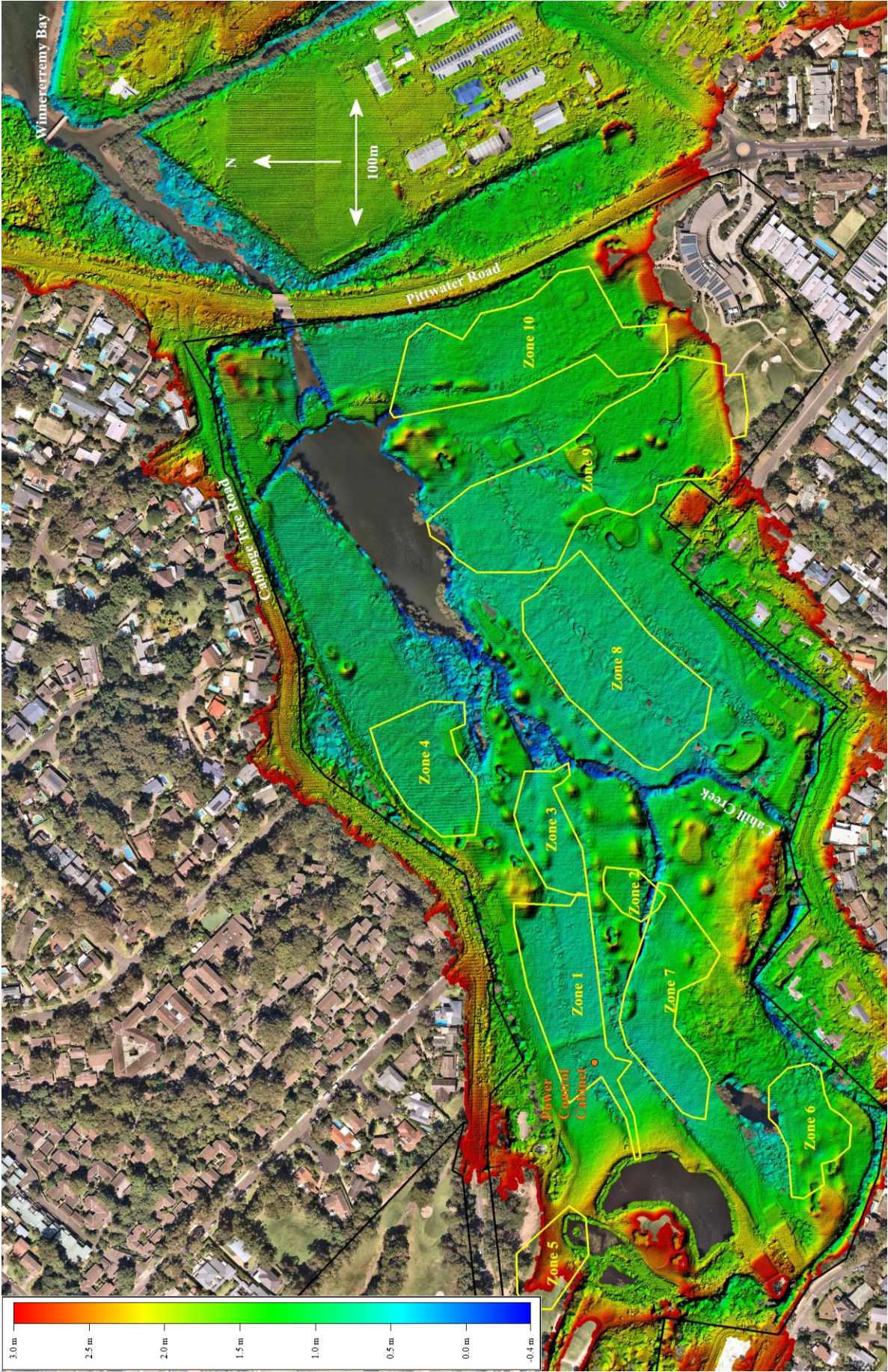
Figure 2: Elevations (up to 3m AHD) over majority of Bayview Golf Club as captured in June 2020
