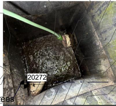
Photo: testing Storm water pit with hose
