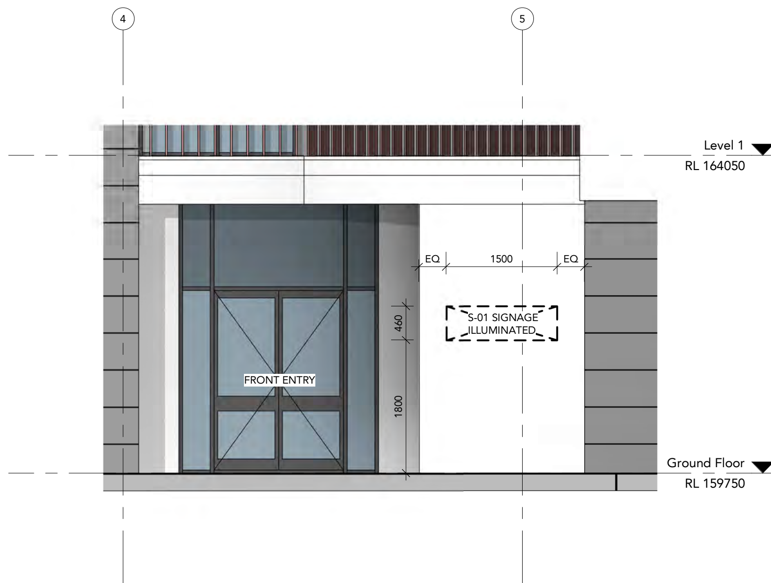
3 West Elevation - Signage Scale: 1 : 50
