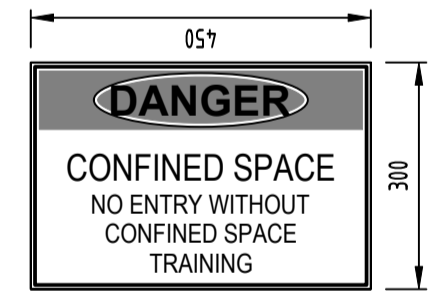
DETAIL CONFINED SPACE SIGN SCALE 1:10
