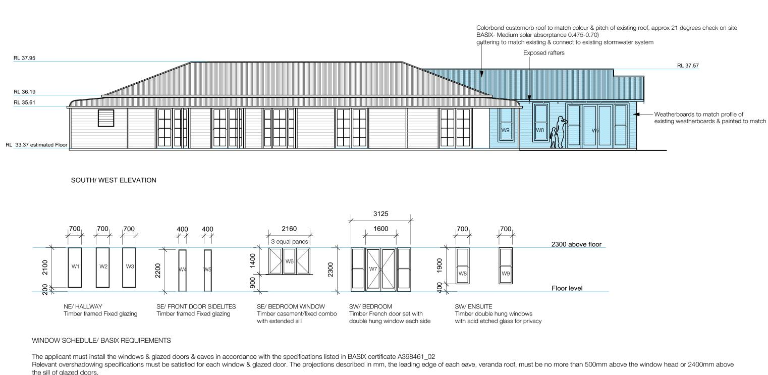
Overshadowing vegetation must be of height & distance from the centre & the base of the window & glazed door as specified in the overshadowing column of Basix certificate.
