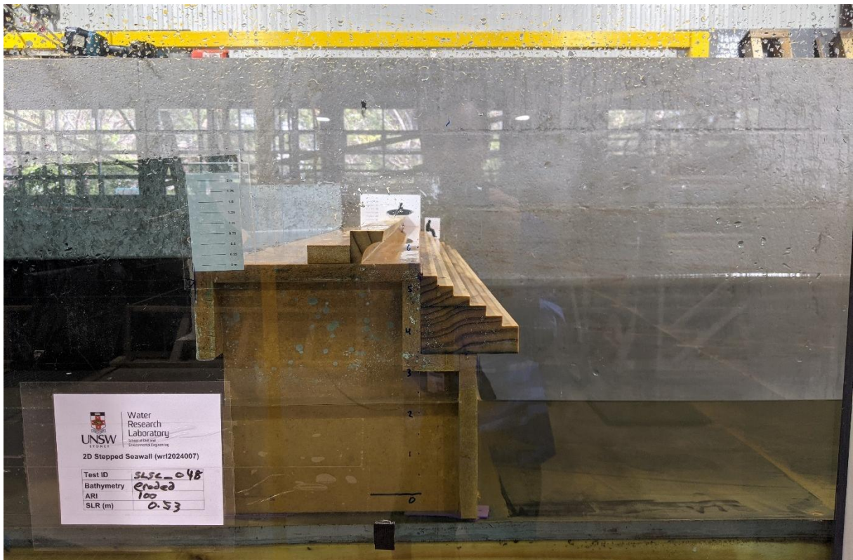
Figure 3.7 Design 1, Original DA seawall (eroded profile), preliminary recurved parapet
