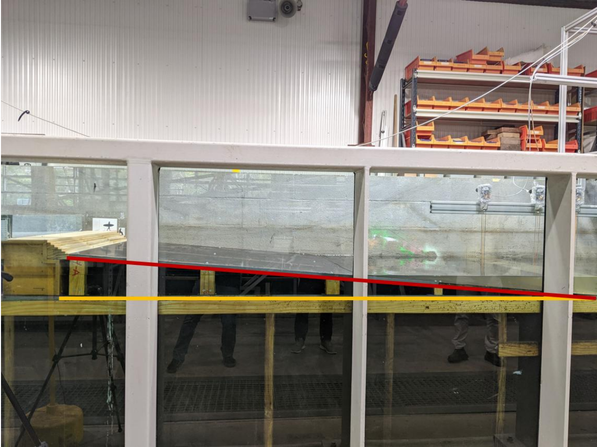
Figure 3.4 Average (red) and eroded (yellow) profiles in flume
