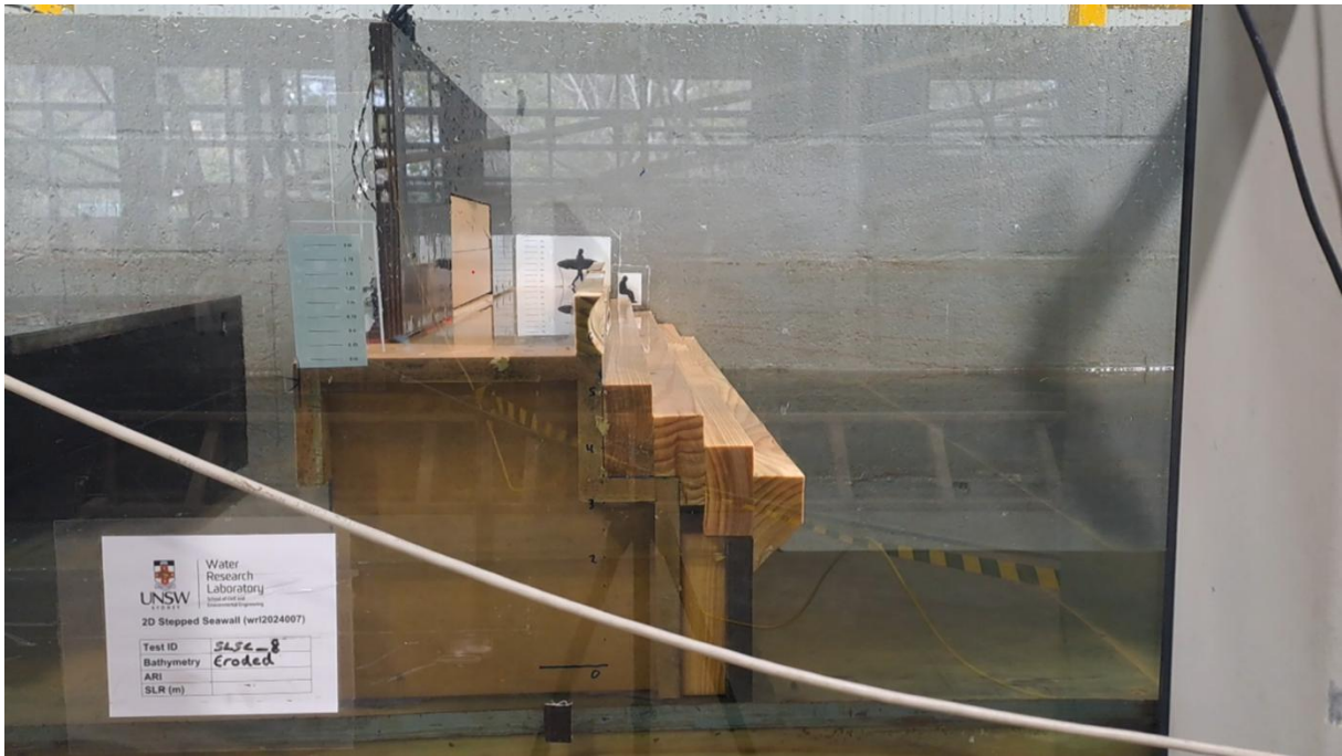
Figure 3.14 Design 4, 4 bleachers and SLSC wall (eroded profile), recurred parapet
