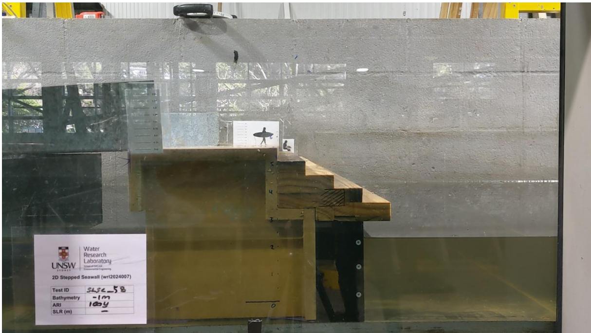
Figure 3.9 Design 2, BCA compliant 4 bleachers seawall (eroded profile)
