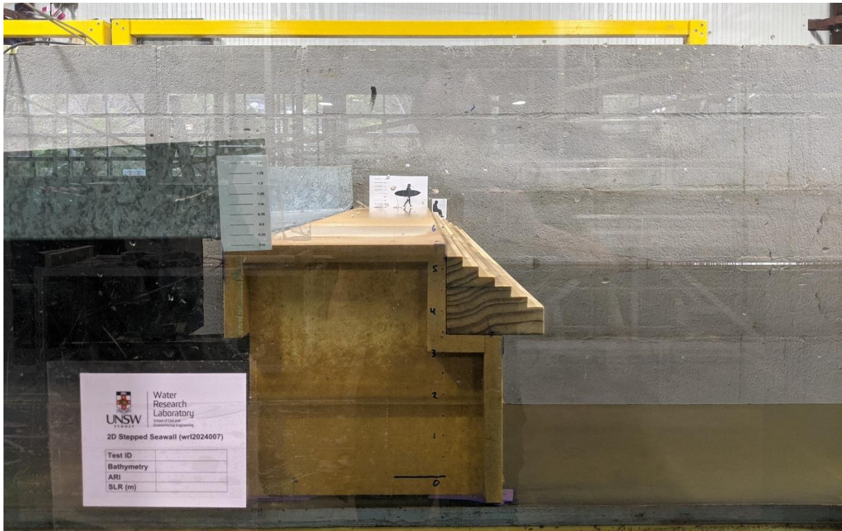
Figure 3.6 Design 1, Original DA seawall (eroded profile)
