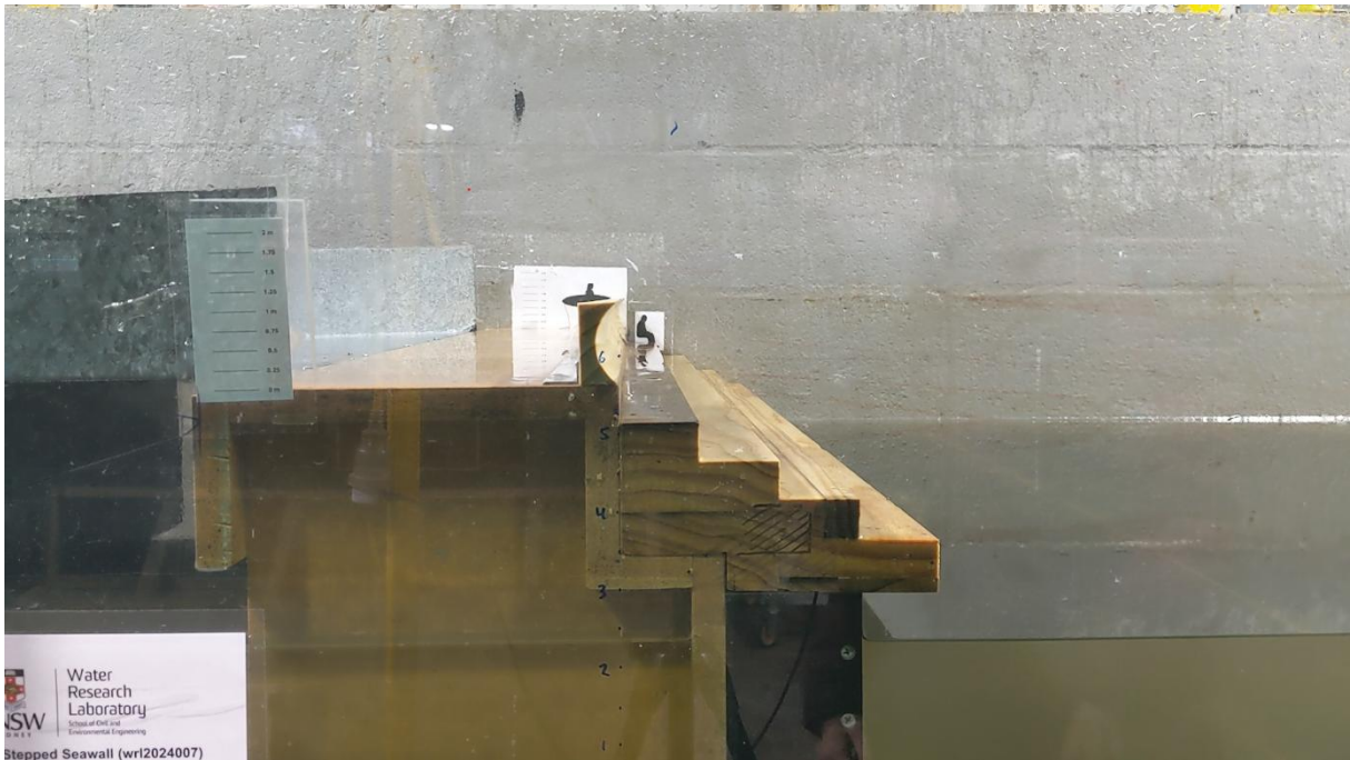
Figure 3.10 Design 2, BCA compliant 4 bleachers seawall (eroded profile), recurved parapet
