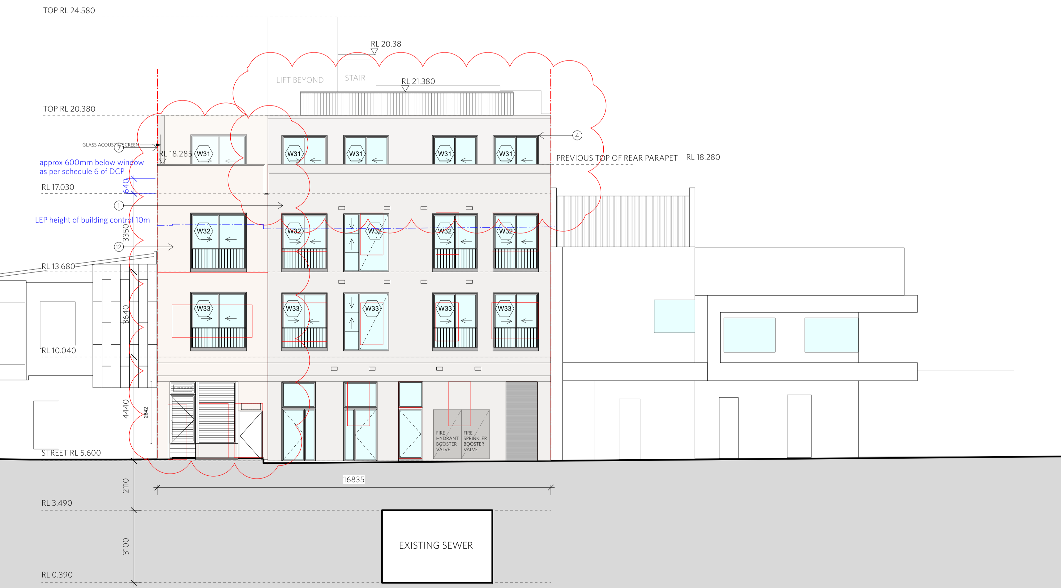
12. Rough Bag Render to the Market Lane facade of No.23 to differentiate it from No. 19-21
