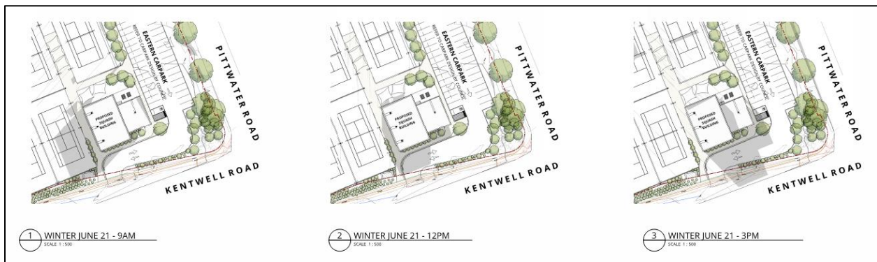
Figure 19. Winter solar access and overshadowing diagram (Source: Webber Architects, 2024)
