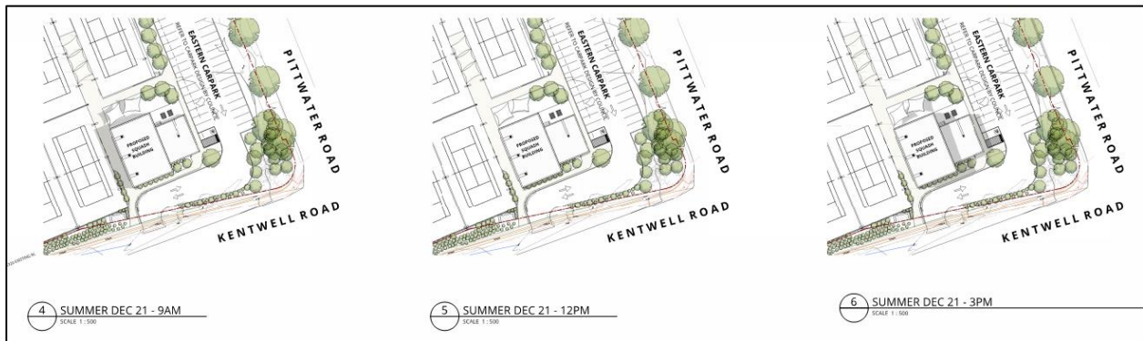
Figure 20. Summer solar access and overshadowing diagram (Source: Webber Architects, 2024)
