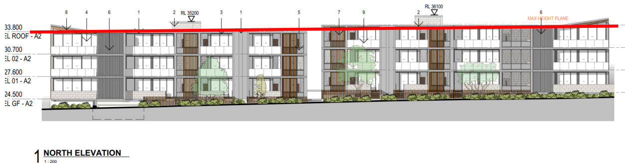
Figure 2 - Diagram showing building height breach along northern façade
