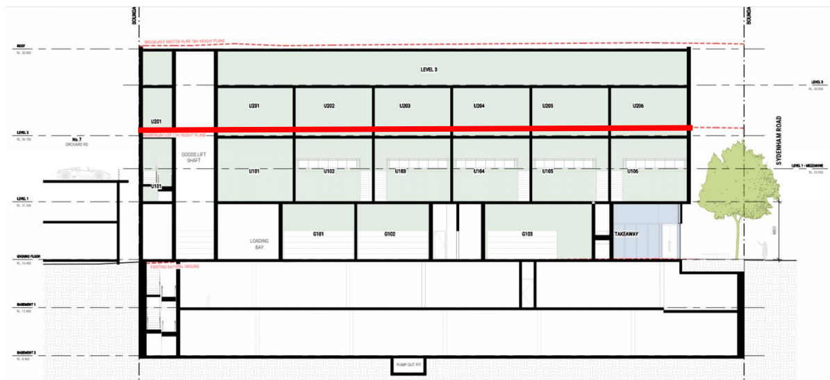
Figure 5 - Plan extract showing extent of building height breach with the red line showing the 11 metre height standard measured above ground level (existing)
