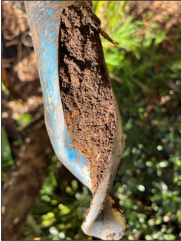
Figure 5. Collection of samples S1, sandy fertile top soil.
