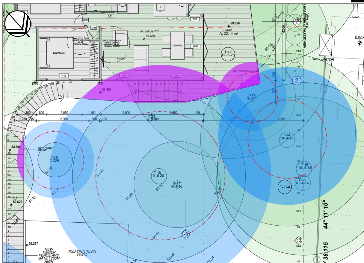
Figure 6 – Tree 13, 14, 18 & 19 – Mark up of Granny Flat Plan, dwg no. A.03, 12/5/23 authored by Gartner Trovato Architects. Red dotted circle notes SRZ, blue shaded circle TPZ, pink shading is encroachment. Marked up by Treeism. NOT TO SCALE.
