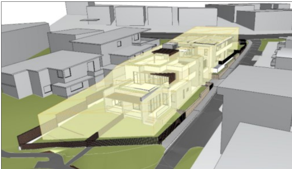
Figure 1 - Envelope Breach at 8m height limit (SEPP HSPD). Source: Cottee Parker Architect
