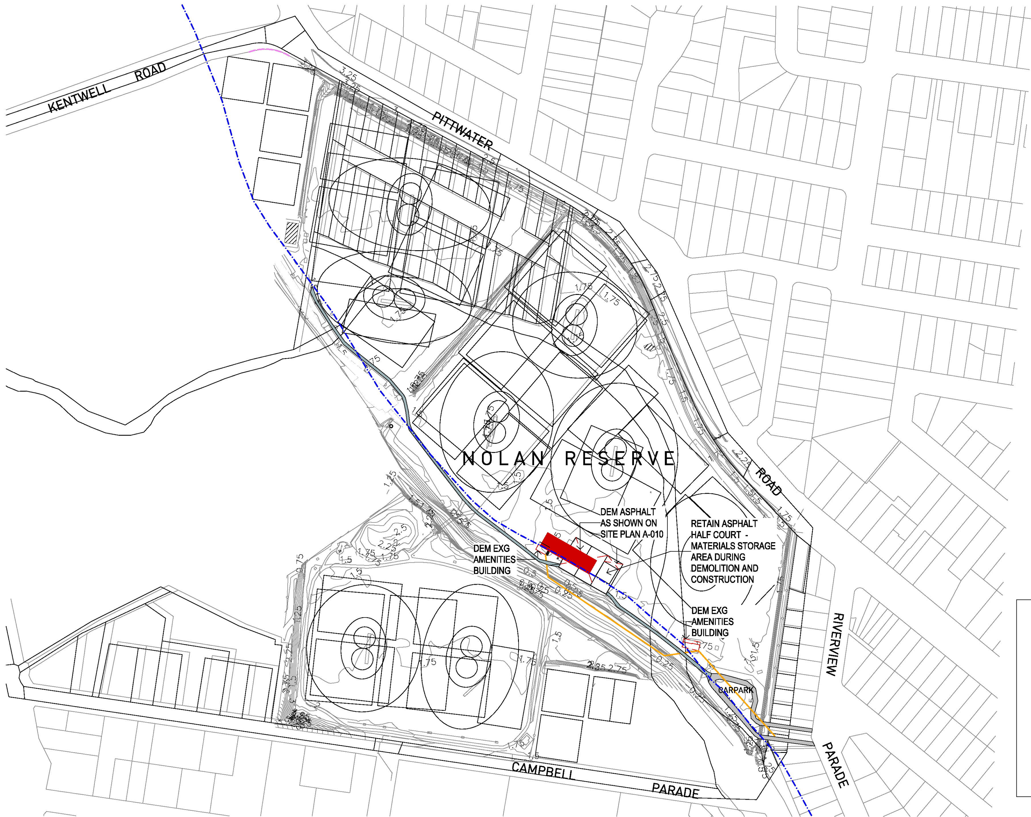
SITE PLAN SHOWING DEMOLITION & WASTE MANAGEMENT 1:2000
