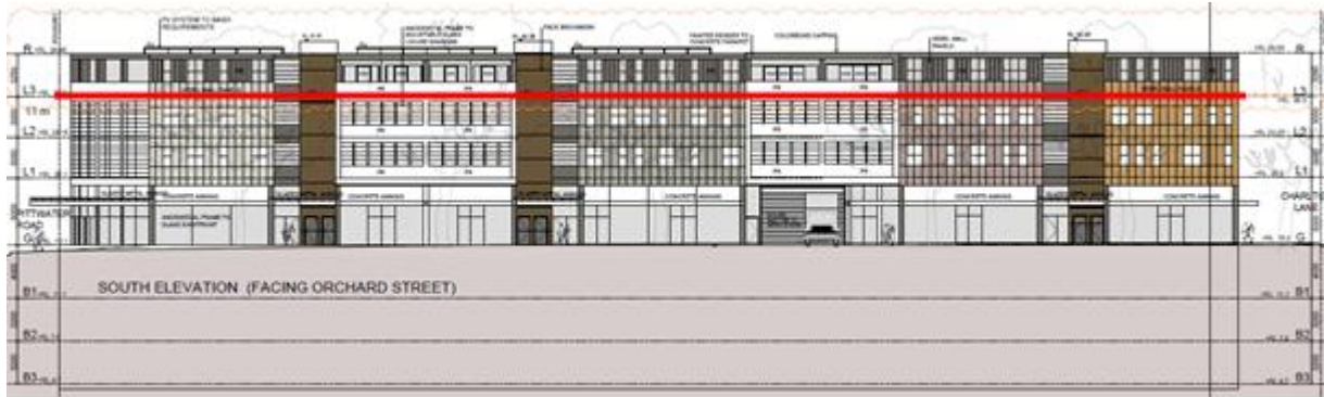
Figure 2 – Plan extract showing extent of 11 metre building height breach southern façade
