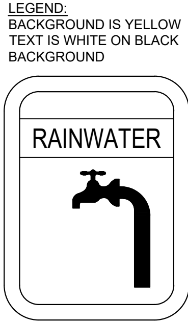
DETAIL 2 RAINWATER SIGN SCALE 1:10
