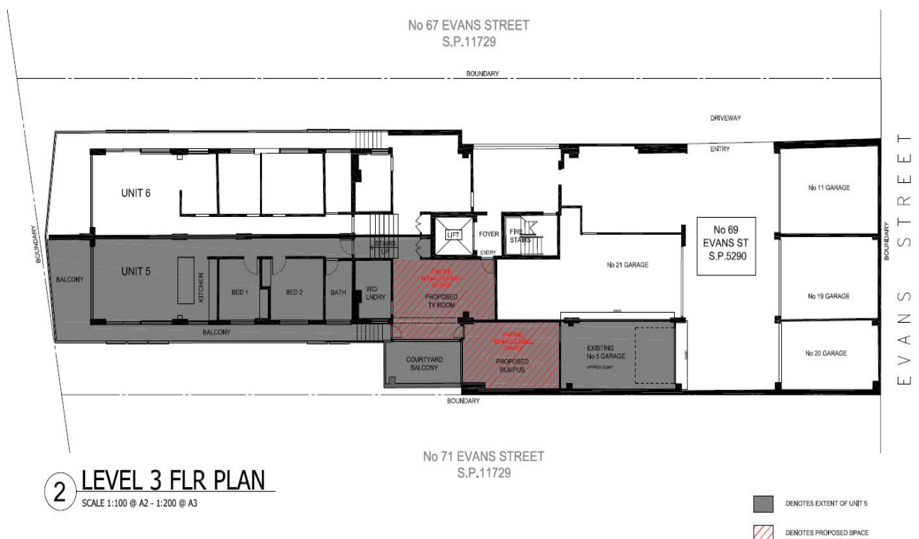
EXISTING LAYOUT PLAN OF UNIT 5 WITH THE PROPOSED CHANGE AREA SHOWN IN RED
