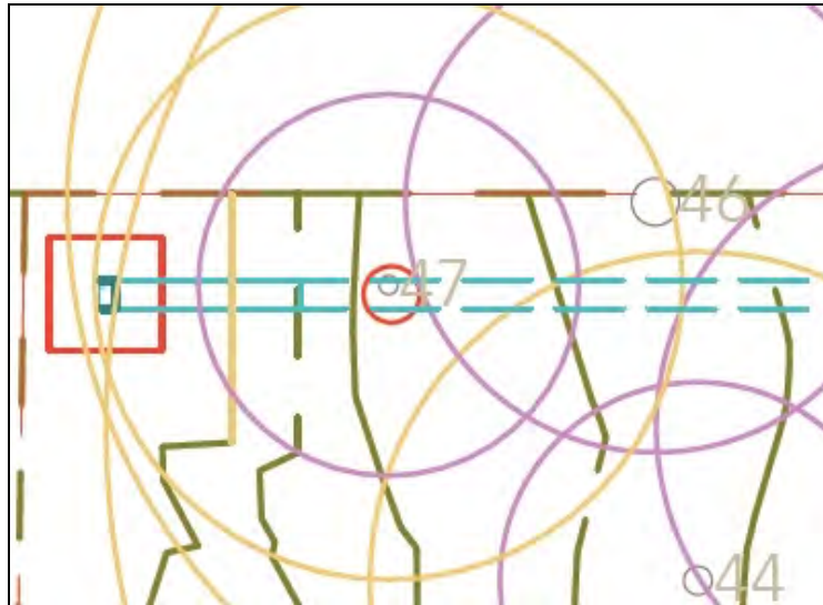
Figure 22: The tree impact plan showing the conflict between Tree 47 and the proposed inclinator path and footing. (Source: Proposed Plans by ANNE ROBSON ARCHITECTURE PTY LTD dated 29/03/2023)
