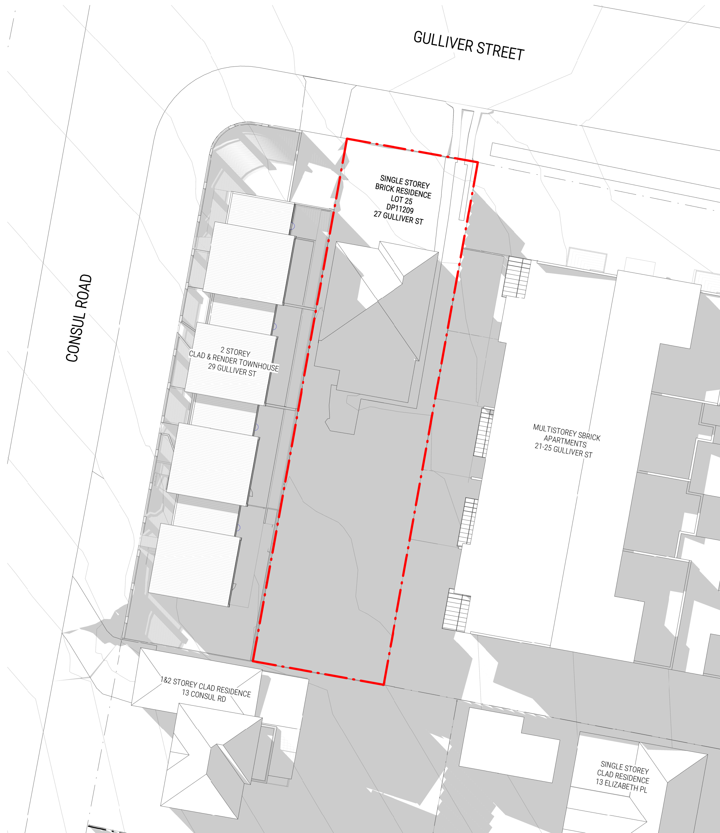
1 EXISTING SHADOW DIAGRAM - 3PM JUNE 21ST DA502/ 1:200 @ A1
