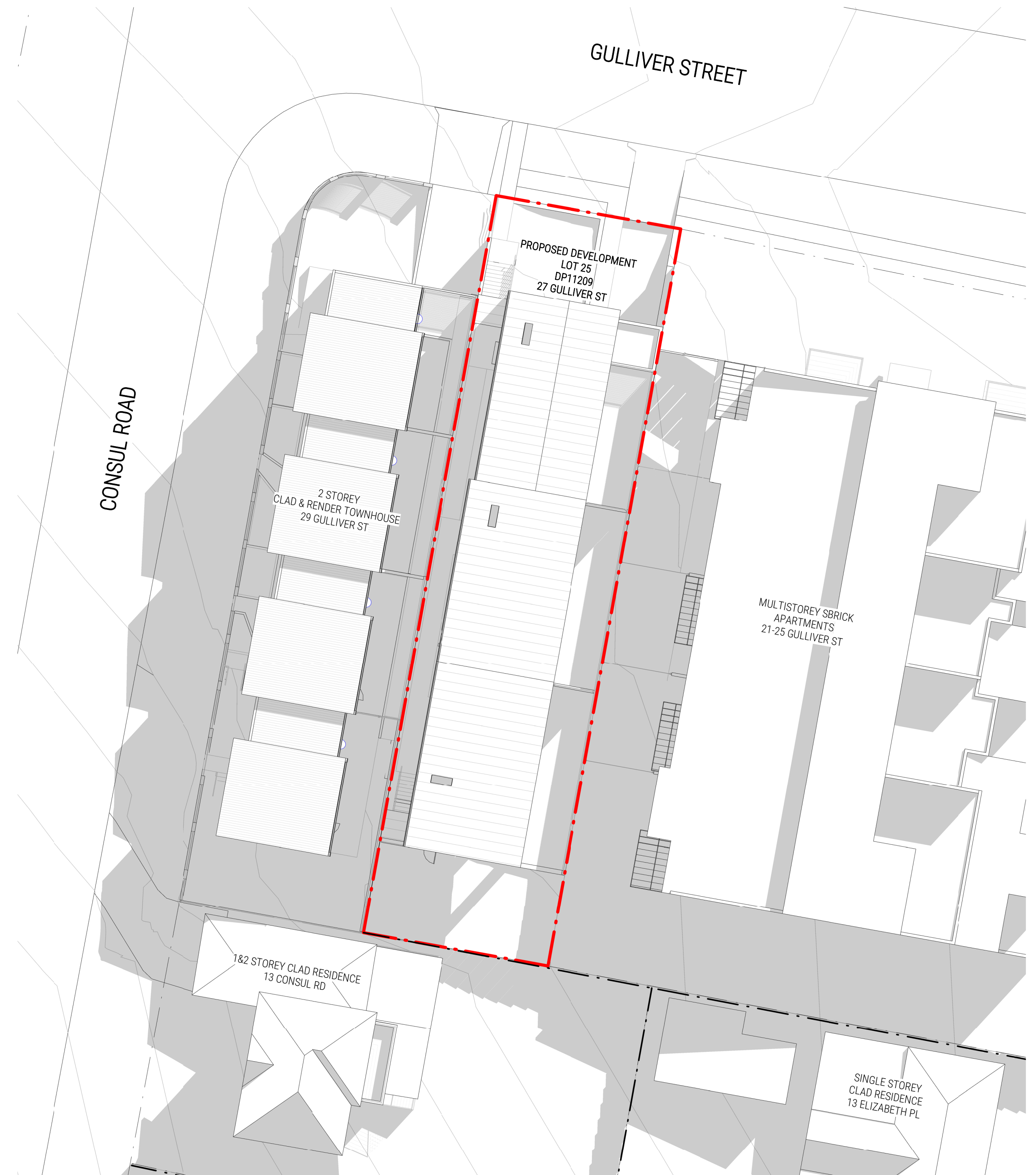
2 PROPOSED SHADOW DIAGRAM - 9AM JUNE 21ST DA500 1:200 @ A1
