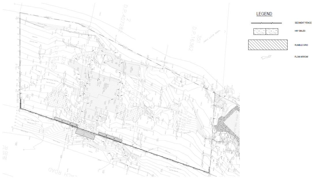
Figure 33: Proposed sediment and erosion control plan (Source: Harris Page and Associates)
