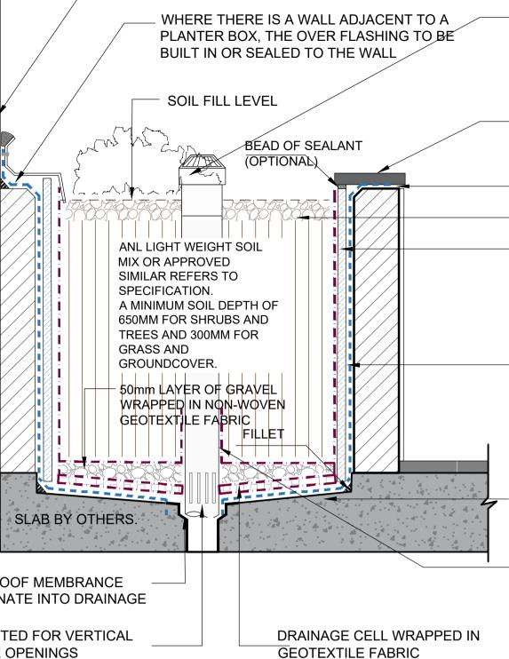
WATERPROOF MEMBRANCE TO TERMINATE INTO DRAINAGE OUTLET PIPE SLOTTED FOR VERTICAL DRAINAGE OPENINGS
