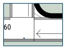
A swinging door in a required exit or forming part of a required exit must not encroach at any part of its swing by more than 500mm impeding the path of travel. The Water Tanks Room door swing opens more than 500mm into the required exit for the basement and therefore is non-compliant in accordance with BCA Clause D3D25.
