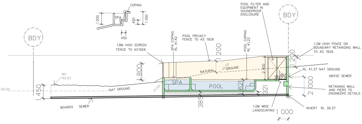
CONCRETE POOL CONSTRUCTION AND PIERING TO SYDNEY WATER REQUIREMENTS TO ENGINEERS DETAILS
