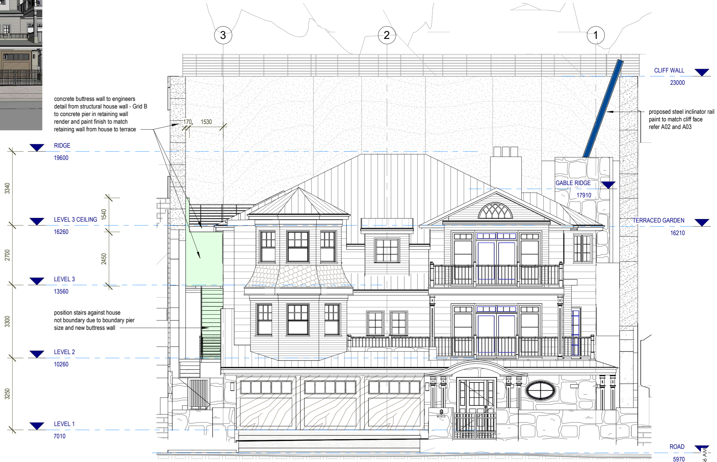
1 EAST ELEVATION - BUTTRESS WALL 1 : 100
