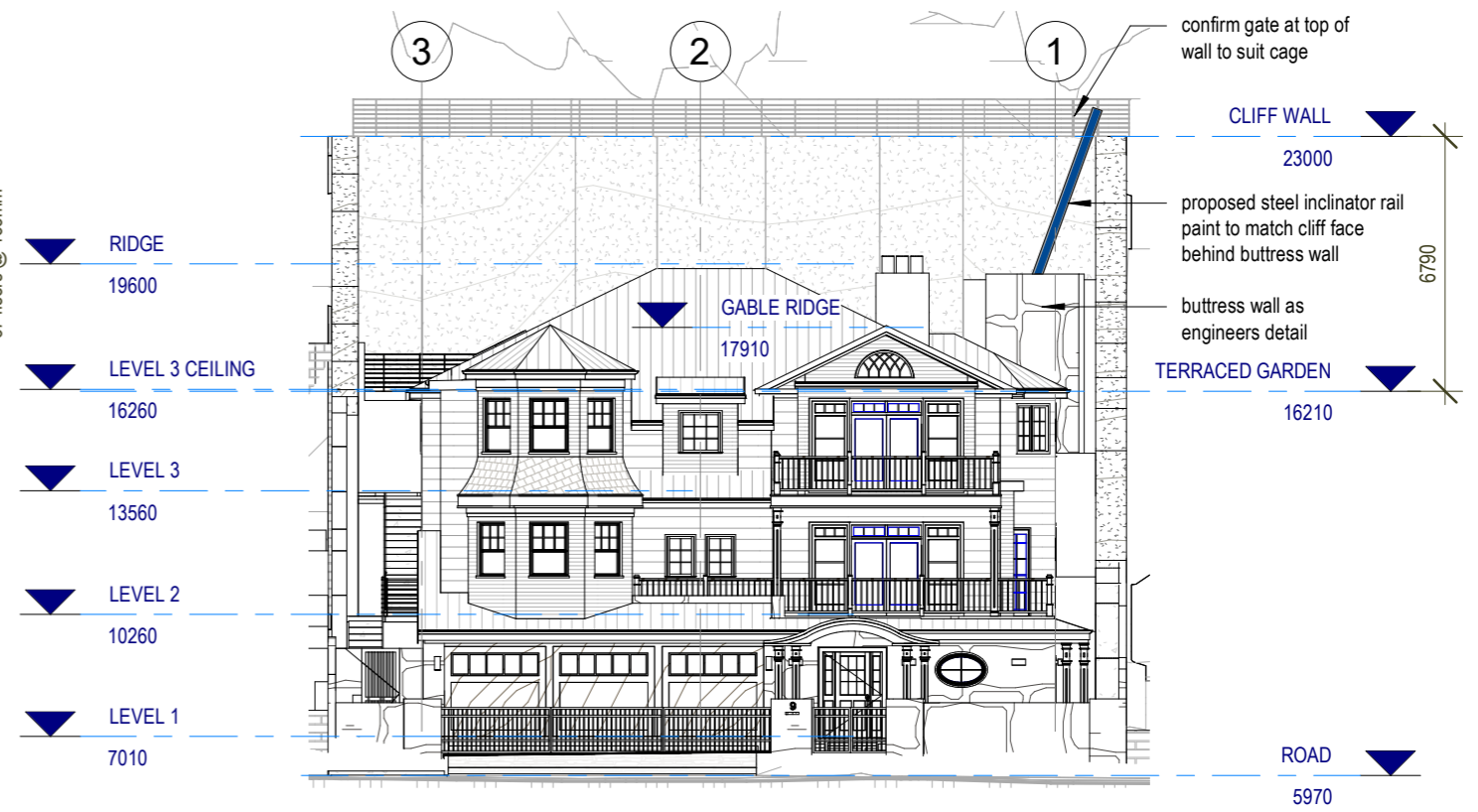
2 EAST ELEVATION - PROPOSED INCLINATOR 1 : 200
