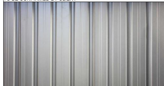
MT-01 PAINTED COLOURBOND METAL ROOF SHEETING. 'IRONSTONE' OR SIMILAR WHERE MARKED ON ELEVATION.
