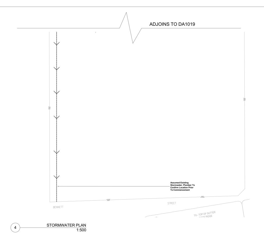
Plumber To Confirm Location Of Existing Stormwater/Sewer Prior To Commencement
