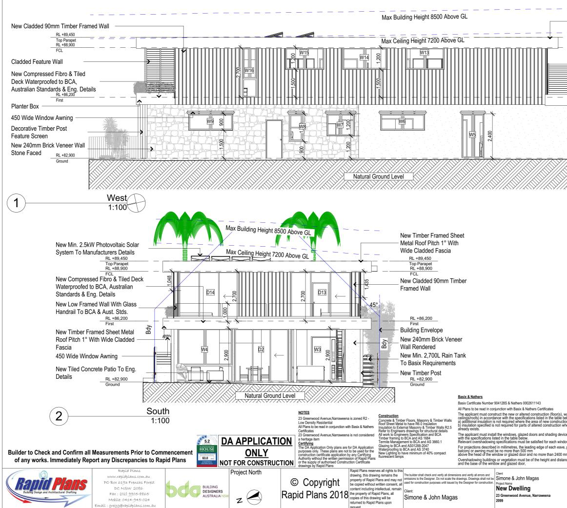
New Timber Framed Sheet Metal Roof Pitch 1° With Wide Cladded Fascia RL +89.450 Top Parapet RL +88,900 FCL New Horizontal Slat Privacy Screen New Timber Framed Sheet Metal Roof Pitch 1° With Wide Cladded Fascia RL +86,200 First New Horizontal Slat Privacy -Screen New Timber Post 10 RL +82,900 ~ Ground 777/////// New 240mm Brick Veneer Wall Rendered
