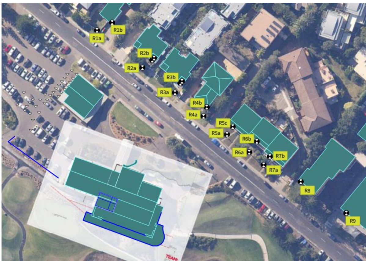
Figure 2. Receiver locations (Image from CadnaA model)
