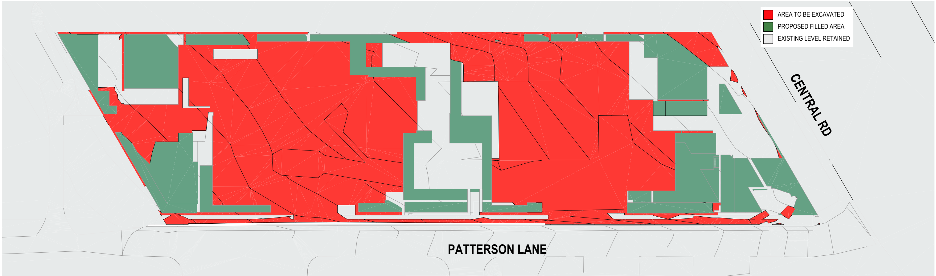
1 - PROPOSED EXCAVATION DIAGRAM - 2D / PLAN SCALE 1:250 @ A3
