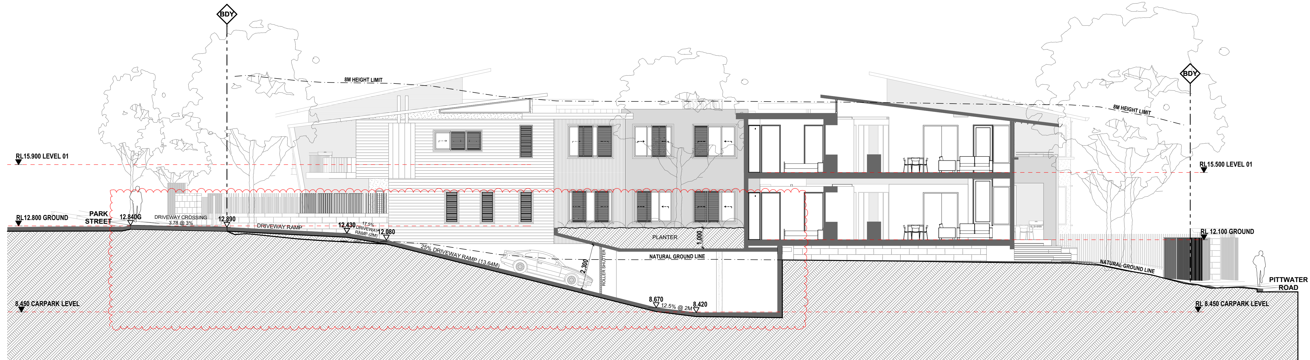
SECTION B (DRIVEWAY RAMP)
