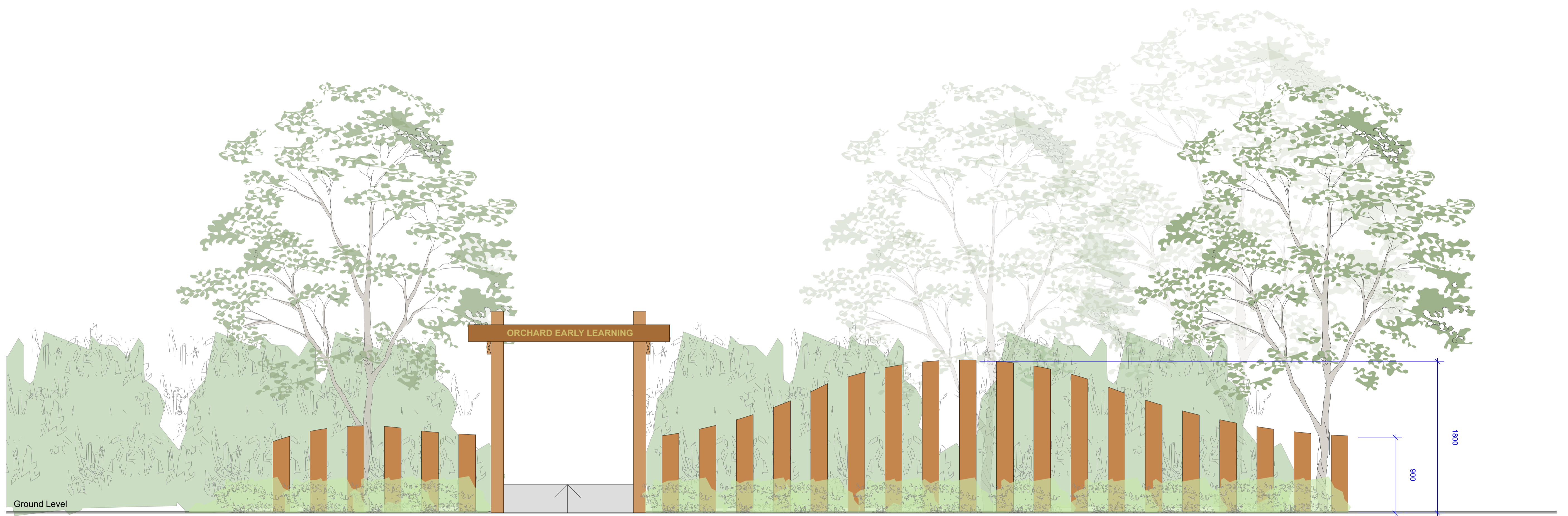
VERTICAL SLEEPER SCREEN ELEVATION 1:25
