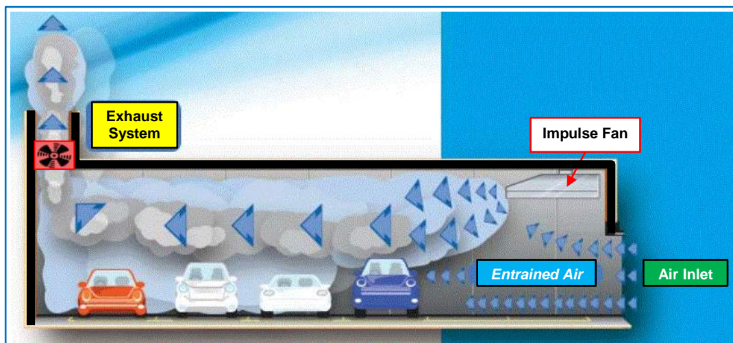
Figure 4: Principle of operation - workings of an Impulse Fan (Image © Fantech)
