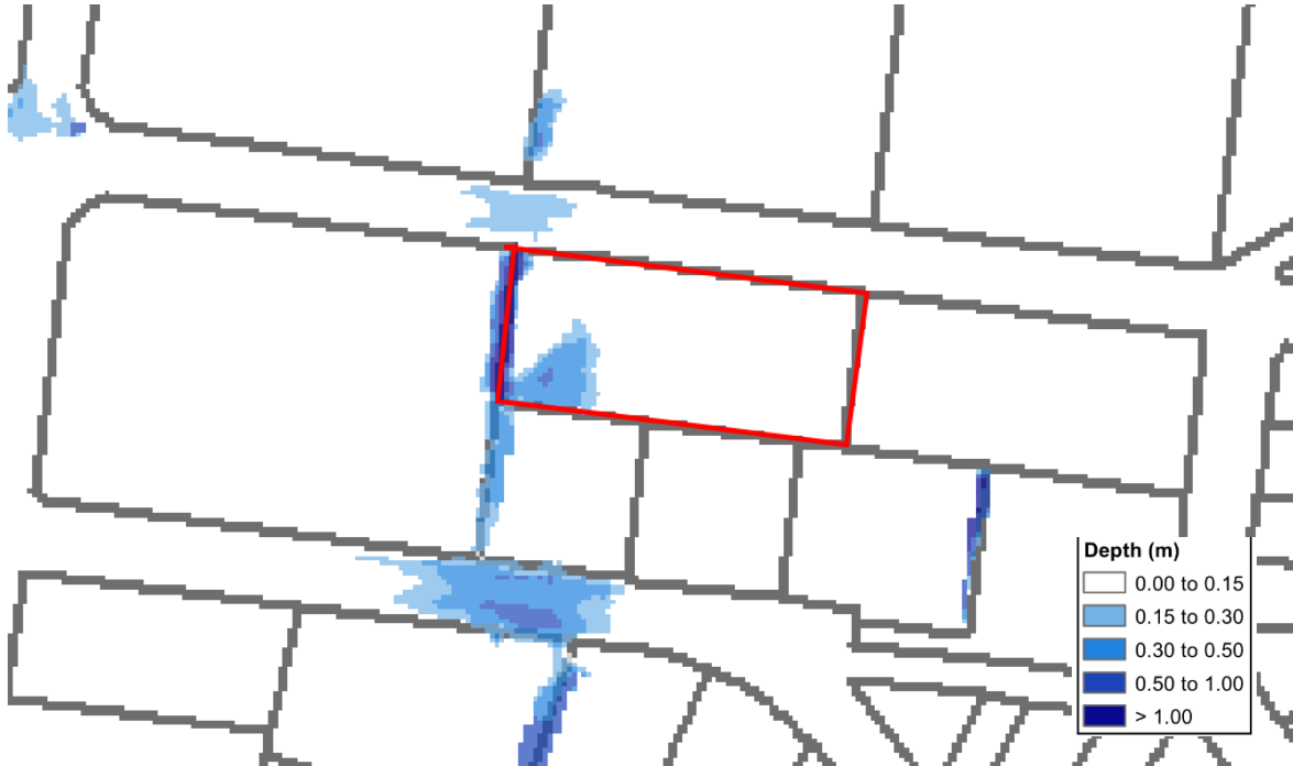
Figure 2 - 20% AEP Flood extent.
