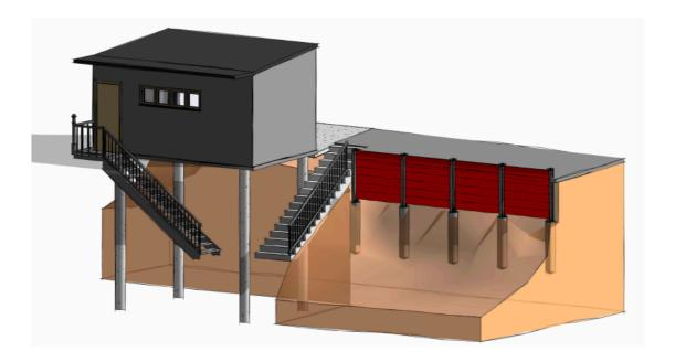
Figure 1: 3D Montage of proposed retaining wall.
