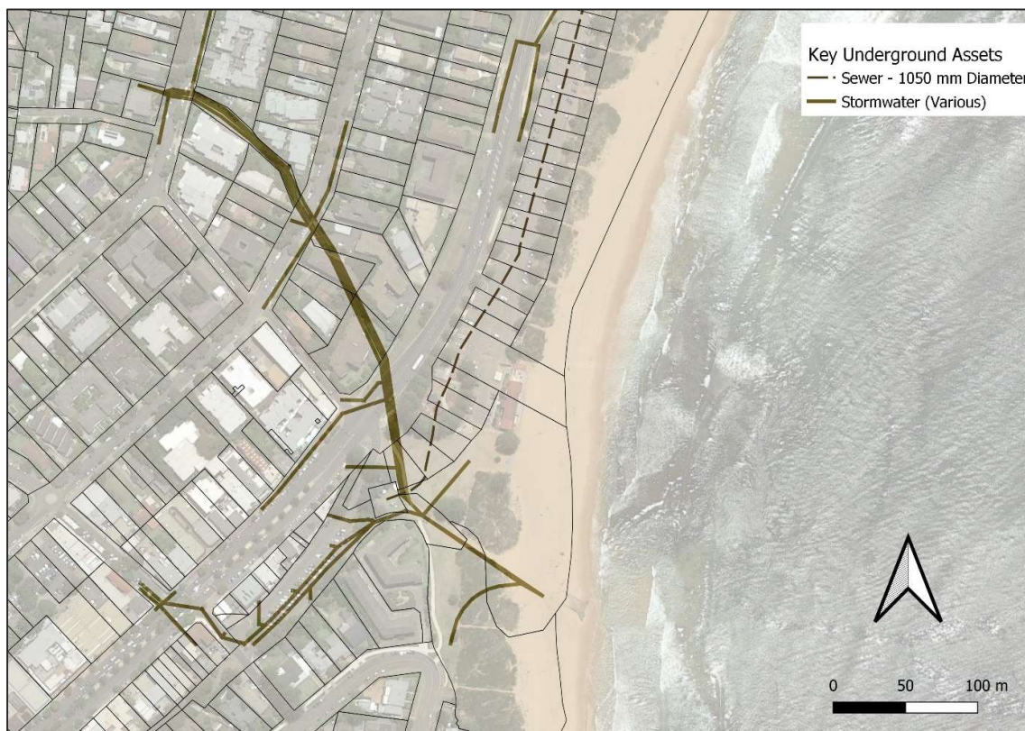
Figure 3-5 Council stormwater and Sydney Water main sewerage line (source: DBYD search 17 November 2022)
